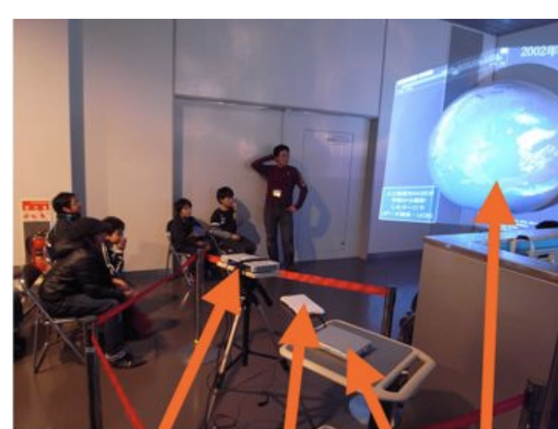
PC projector Balance Wii board 2-m Spheric Screen (balloon)
