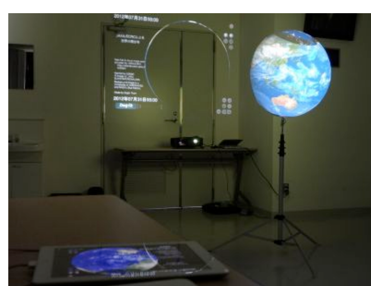
Both side projection with two projectors
